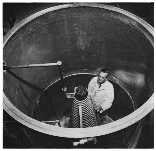
CHUCK THACKER (5312) inspects a carbon/carbon cone prior to chemical vapor deposition process inside a huge furnace in Bldg. 845. The piece is subjected to temperatures up to 2000°F in a methane-argon atmosphere.
